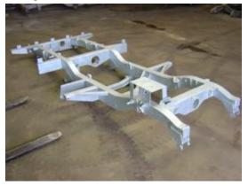
Fig:. Ladder Frame Chassis
