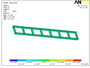
Fig. SHEAR STRESS IN XY
